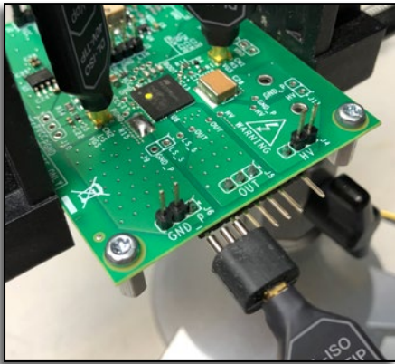
DL-ISO with flexible interfaces to DUTs
