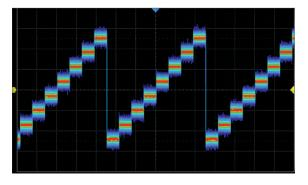
The Color temperature display clearly shows noise and jitter with infrequently occurring waveforms shown in blue through to the most frequently occurring waveforms shown in red.
