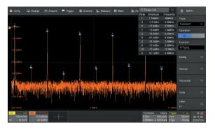
Two Math traces support Plus, Minus, Multiply, Divide, FFT, integration, differential, square root, average, Eres and formula editor, providing a quick insight into the waveform characteristics.
