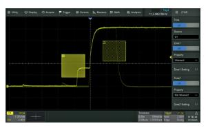
Set up to 2 zones defining each as either an Intersect or a Non Intersect. Trigger occurs when conditions are met. Zone Trigger helps to simplify advanced triggering.
