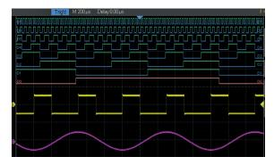
The MSO option adds 16 digital channels to the T3DSO3000 enabling users to trigger and acquire digital as well as analog waveforms in a mixed signal debug environment.
