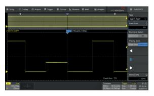
The T3DSO3000 can find events within an acquisition record or history acquisition based on user specified trigger conditions. Navigate browses through Events flagged by the Search, plays back history events or continuously moves the delay position on long records (useful in zoom view).
