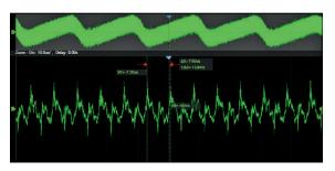
The record length of up to 250 Mpts (interleaved) or up to 125 Mpts (non-interleaved) allows use of a higher sampling rate to capture more signal detail. The hardware-based Zoom then allows quick zoom in to any area of interest.
