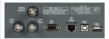
Connectivity includes External Trigger Input, Pass/Fail and Trigger Out, USB Device (USBTMC) and LAN for remote control, and a Kensington Lock security point.
