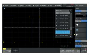
The always enabled History mode records up to 100,000 waveforms allowing users to scroll back through previous acquisitions to analyze past events and locate anomalies quickly. Serial decode, zoom and cursor measurements can be used.
