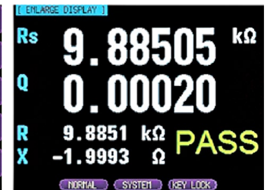
ENLARGE Display Enlarge Measurement Results and Include PASS/FAIL Result
