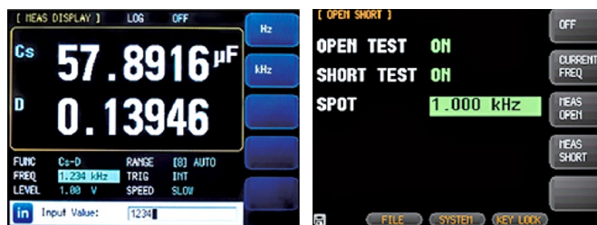
Continuous and Adjustable Frequency Freely Input Frequency Within Provided Frequency Range
