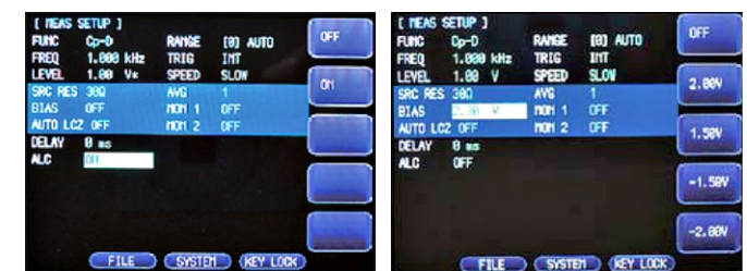
Automatic Level Control Ideal for Measuring Components With Specific Voltage Requirements
