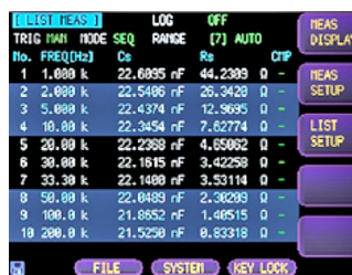
Listed Tests Variation Criteria Based on Frequency or Voltage/Current
