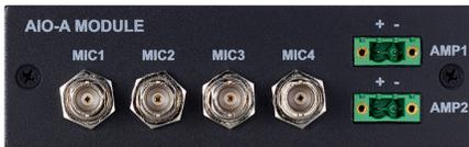
**A Acoustic:** Four mic/line inputs with CCP, TEDS; two 10 W class-D amplifier outputs.
