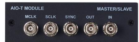
**T TDM:** Digital TDM, up to 10 channels, 24 or 32 bit samples, 192 kHz.
