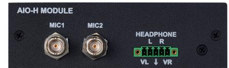
**H Headphone:** Two mic/line inputs with CCP, TEDS; two headphone/earbud outputs with impedance measurement.
