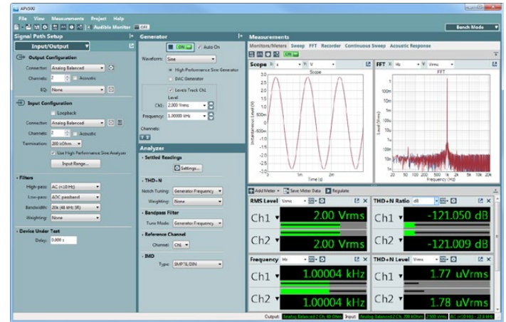
APx500 Bench Mode, showing live meters and monitors for waveforms, FFT, RMS levels, frequency and THD+N.
